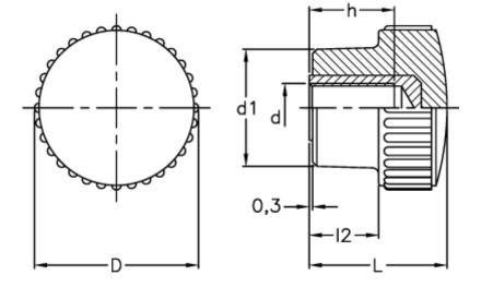
$$\begin{array}{ll} D & = 26 \\ d1 & = 16 \\ d \ 6H = M8 \\ h & = 20 \\ L & = 28 \\ l2 & = 15 \end{array}$$
